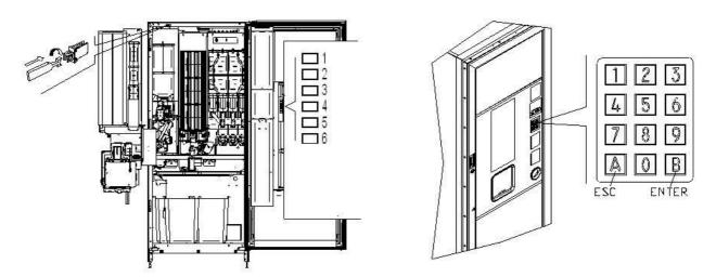
**Programming Button:** once programming is accessed, **Command 00** appears on the display. Direct access is possible from this main menu to several data or other submenus. Enter the command on **Direct selection keypad** and press **key ENTER** to confirm the selection.
